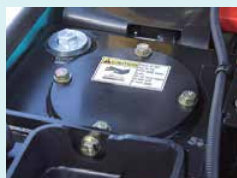
Hydraulic oil tank
