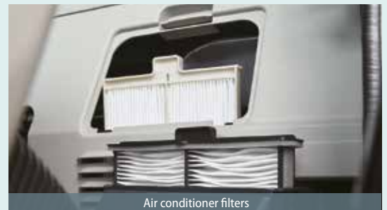
Air conditioner filters
