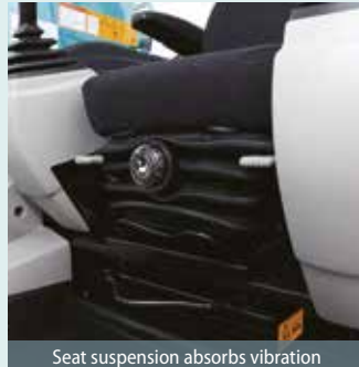
Seat suspension absorbs vibration
