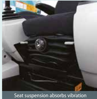
Seat suspension absorbs vibration
