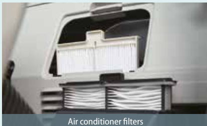
Air conditioner filters
