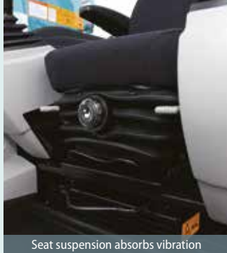
Seat suspension absorbs vibration
