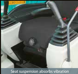
Seat suspension absorbs vibration
