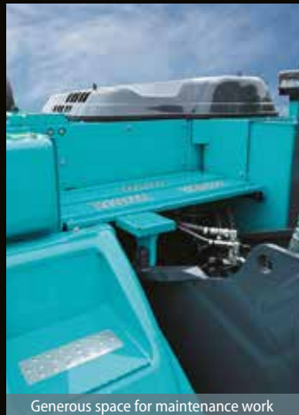
Generous space for maintenance work
