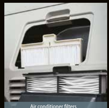
Air conditioner filters
