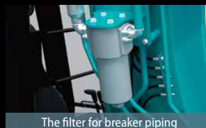
The filter for breaker piping
