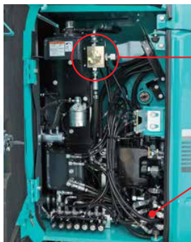
Easy access to main control valves
