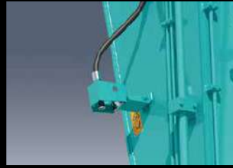
Water spray piping Water spray piping with two-nozzle is provided on both the upper section and the right side of the arm.
