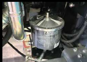
Case drain filter A first for the class, a hydraulic case drain filter is equipped for improved filtration and reliability.
