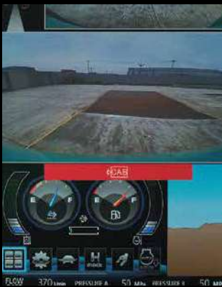
Cab interference warning display
