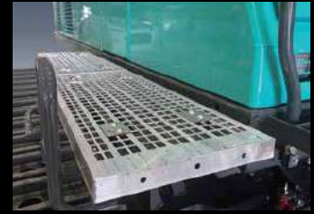
Removable walkway Walkways are provided on both the left and right sides of the base of the machine, allowing easier access for maintenance.
