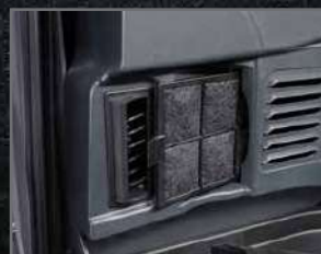
Air conditioner filter for internal air circulation
