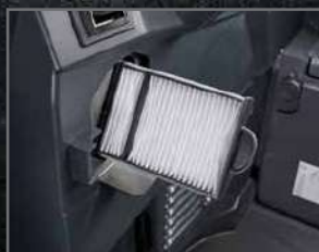
Air conditioner filter for outer air intake
